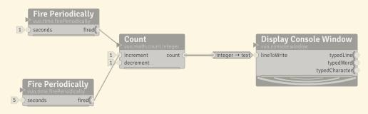
On some nodes, like **Count**, the receptor port lets you bypass the work typically done by the node and just conduct the event. For example, this graph shows how you can use the receptor port to get the **Count** node's current count without incrementing or decrementing it.
