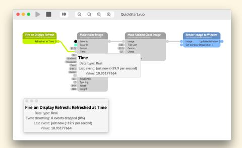
As you can see, the events and data shown in the two port popovers are the same. A stream of information is flowing out of the **Refreshed at Time** output port, along the cable, and into the **Time** input port.
