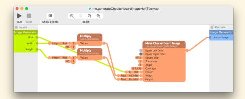
To fix the composition above, you could add an event cable from the **time** published input port to each of the **Multiply** nodes. This would ensure that the **Multiply** nodes provide the halved width and height to **Make Checkerboard Image** whenever **Make Checkerboard Image** needs them, even if **width** and **height** have constant values.
