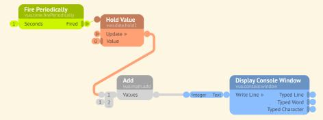
This composition uses a feedback loop to keep track of a count, which it prints upon a console window: 1, 2, 3, 4, . . .
