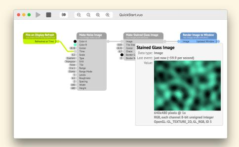
Now that the Fire on Display Refresh, Make Noise Image, and Make Stained Glass Image nodes have worked together to produce the image shown in the port popover, the final step is for the Render Image to Window node to display the image in a window.
