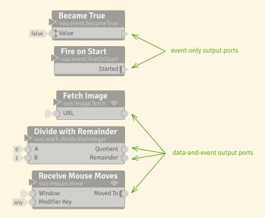
**3.2.2.1 Trigger ports** Although trigger ports can *create* events, they never *transmit* events that came into the node through an input port (hence the thick line to the left of each trigger port — an event wall), nor do they cause any other output ports to emit events.
