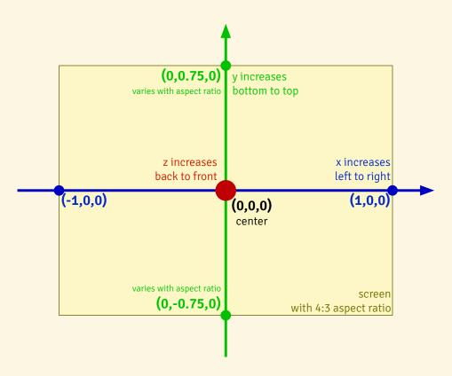
Typically, as illustrated above, the position (0,0) for 2D graphics or (0,0,0) for 3D graphics is at the center of the rendering area. The X-coordinate -1 is along the left edge of the rendering area, and the X-coordinate 1 is along the right edge. The rendering area's height depends on the aspect ratio of the graphics being rendered, with the Y-coordinate increasing from bottom to top. In 3D graphics, the Z-coordinate increases from back to front.
