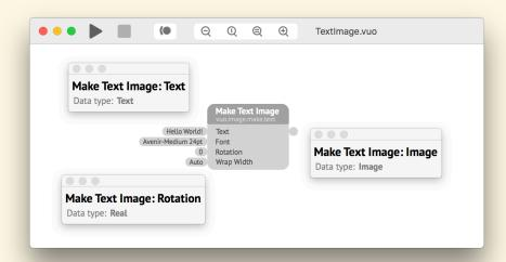
When you start dragging a cable from a port, Vuo shows you which ports you can connect the other end of the cable to — ports that have a compatible data type — by fading out all other ports. Ports that remain opaque have the same data type as the original port. Ports that are slightly faded have a data type that is different but related, so it's possible to convert from one data type to the other.
