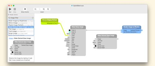
Draw a cable from the Make Noise Image node's output port to the Make Stained Glass Image node's Image input port, then another cable from the Make Stained Glass Image node's output port to the Render Image to Window node's input port.
