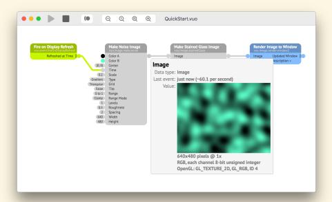
Each time the **Make Noise Image** node does its job, it sends two pieces of information through its output port — the same event that came in the **Time** input port, accompanied by new data: the image created by the node.
