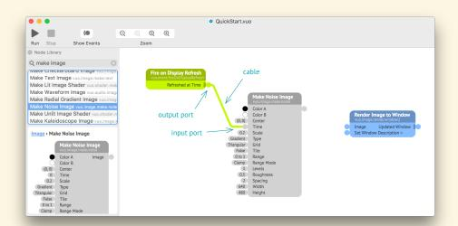
Next, drag a cable from the output port of **Make Noise Image** and drop it on the **Render Image to Window** node's **Image** input port.
