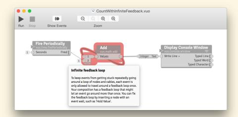
The above composition is an example of an infinite feedback loop. Any event from the Fire Periodically node would get stuck forever traveling in the feedback loop from the Add node's Sum port back to the **Item 1** port. Because there's no event wall in the feedback loop, there's nothing to stop the event. Every feedback loop needs a node like **Hold Value** to block events from looping infinitely.
