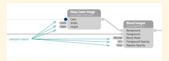
For many data types, the constant value is displayed alongside the input port. You can double-click on the constant value to open an **input editor** and edit the value.
