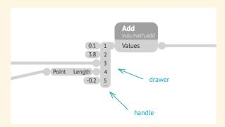
You can change the number of list items by dragging the drawer's handle (bar along the bottom) up or down, or by right-clicking on the drawer and selecting Entfernen Sie den Eingangsanschluss or Eingabeport hinzufügen].
