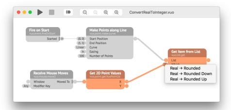
Vuo inserts the type-converter node in a collapsed form to save space. You can still click on the node to see its uncollapsed form and description in the Node Documentation Panel.
