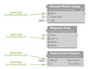
The composition below, Select Movie (File Open Example vuo.select), demonstrates one way that event doors can be useful. This composition displays one of two movies at a time, switching between them each time the mouse is pressed. The doors on the **Select Input** node's **False Option** and **True Option** input ports allow the node to let the stream of events and video frames from one movie through while blocking the stream from the other movie.
