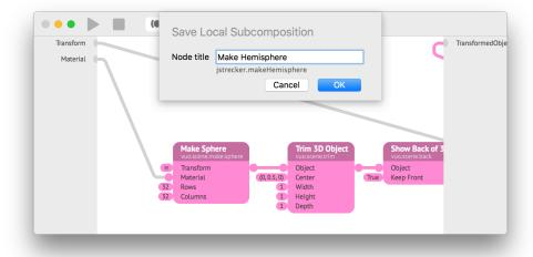
Having named the subcomposition, you now have two windows: one with the subcomposition and one with the original composition, in which the selected part has been replaced with a subcomposition node.
