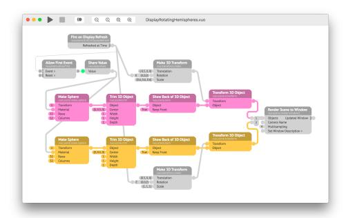
The composition above renders two rotating hemispheres to a window. (The **Trim 3D Object** node cuts off half of the sphere. The **Show Back of 3D Object** node makes the inside of the sphere visible.)
