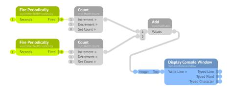
In this composition, the **Add** node executes each time either **Fire Periodically** node fires an event. If one of the **Add** node's inputs receives an event, it doesn't wait for the other input. It goes ahead and executes.
