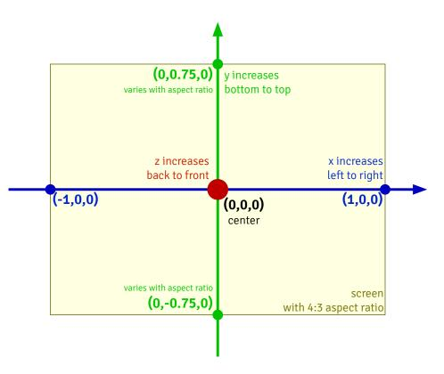
Typically, as illustrated above, the position (0,0) for 2D graphics or (0,0,0) for 3D graphics is at the center of the rendering area. The X-coordinate -1 is along the left edge of the rendering area, and the X-coordinate 1 is along the right edge. The rendering area's height depends on the aspect ratio of the graphics being rendered, with the Y-coordinate increasing from bottom to top. In 3D graphics, the Z-coordinate increases from back to front.
