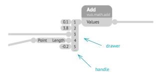
You can change the number of list items by dragging the drawer's handle (bar along the bottom) up or down, or by right-clicking on the drawer and selecting Remove Input Port or Add Input Port.
