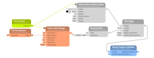
**Count within Range** is one of many ways to cycle through a series of numbers. Another is the **Curve** node when its **Loop** port is set to *Loop* or *Mirror*. And another is the **Wave** node. The composition below (File) Open Example vuo.motion Wave Circle) uses the **Wave** node to make a circle move back and forth.
