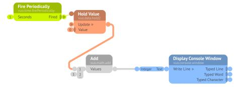
This composition uses a feedback loop to keep track of a count, which it prints upon a console window:  $1, 2, 3, 4, \ldots$
