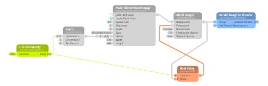
This works. An event from the **Fire Periodically** node travels through the **Count** node to the **Make Checkerboard Image** node, to the **Blend Images Node**. The same event travels through a separate cable to the **Hold Value** node, and then to the **Blend Images** node. There the two events are joined.
