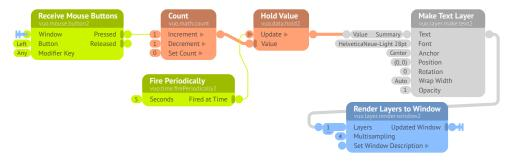
The key to this composition is the **Hold Value** node. Each time the **Count** node outputs a value, the **Hold** Value node holds on to it (in other words, stores it). Every 5 seconds, an event from Fire Periodically hits the Hold Value node's Update port, and the Hold Value node outputs the count that it's storing.
