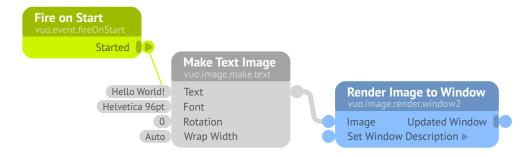
The lines connecting the nodes are called **cables**. Cables are the conduits that data and events travel through.
