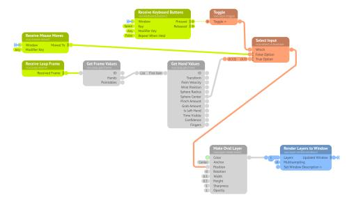
Instead of taking multiple event streams and picking one to let through, as in the previous example, what if you have a single event stream and want to pick one of several downstream paths to route it to? Below is an example of that. The space bar toggles between two circles. Whichever circle is chosen at a given time is controlled by the mouse. This works because the Select Output node routes the data-and-event stream from **Receive Mouse Moves** through just one of its output ports at a time.
