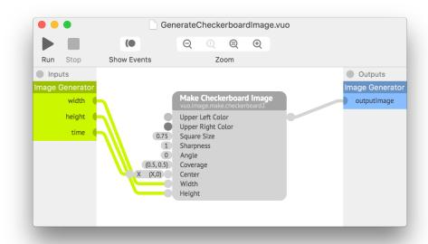
Above is an example of a composition with published ports: Generate Checkerboard Image (File Open Example) Image Generators). It inputs events and data through published input ports called width, height, and time. It outputs events and data through a published output port called outputImage.
