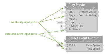
An **input port** is the location on the left side of the node where you can enter data directly, connect a data-and-event cable, or connect an event-only cable. When an event arrives at an input port, it causes the node to execute and perform its function based on the data present at the node's input ports.
