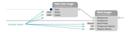
For many data types, the constant value is displayed alongside the input port. You can double-click on the constant value to open an **input editor** and edit the value.
