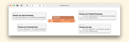
You can connect a generic port to any port that has a compatible data type (which may be either generic or non-generic). When you start dragging a cable, Vuo fades out the incompatible ports, so you can easily see which ports it's possible to connect to.
